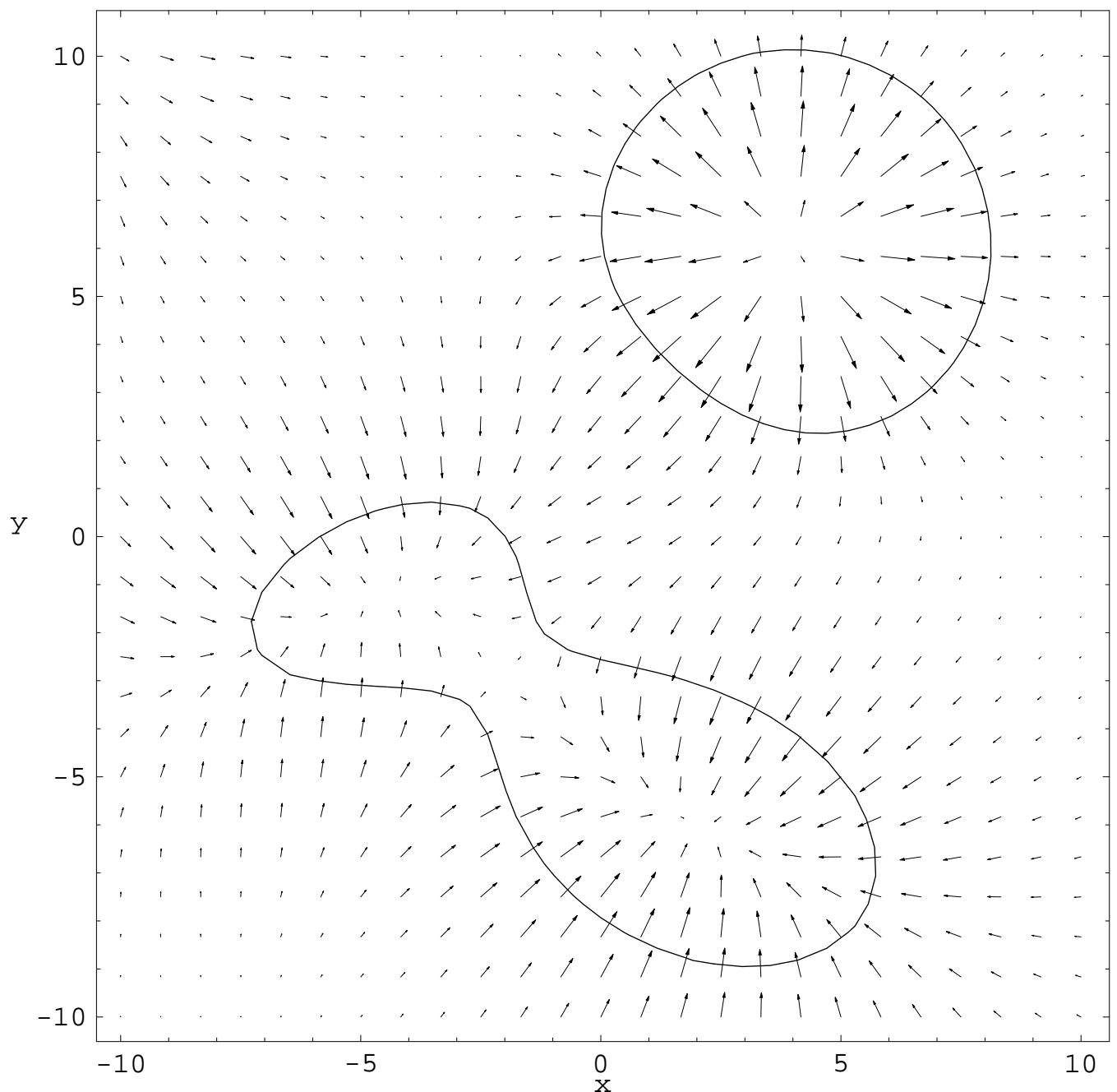
The next figure shows the path of steepest ascent starting at  $(2, 6)$ . Note the similarity to the solution drawn on the board in class.
